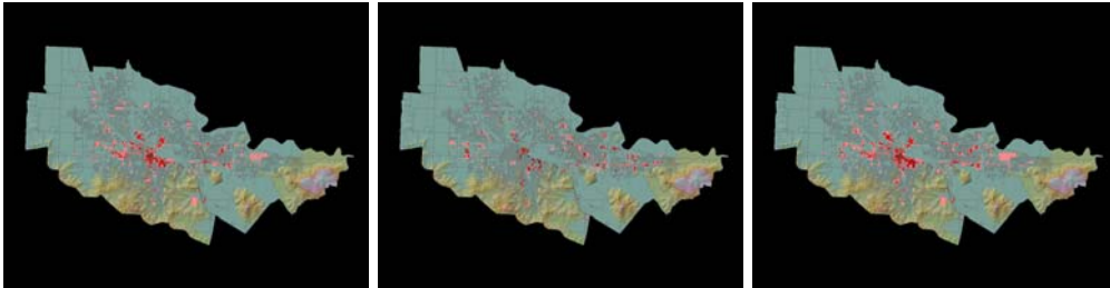
Figure 3. Results from UrbanSim for Eugene/Springfield, Oregon, forecasting land use patterns over a 14-year period. These results arise from the simulated interactions among demographic change, economic change, real estate development, transportation, and other actors and processes in the urban environment. Map (a) shows the employment density in 1980 (number of jobs located in each 150x150 meter grid cell). Darker red indicates higher density. Map (b) shows the predicted change from 1980 to 1994 (where darker red indicates a greater change), and map (c) the predicted employment density in 1994. In a historical validation of the model, this result was then compared with the actual 1994 employment, with a 0.917 correlation over a 1-cell radius.
